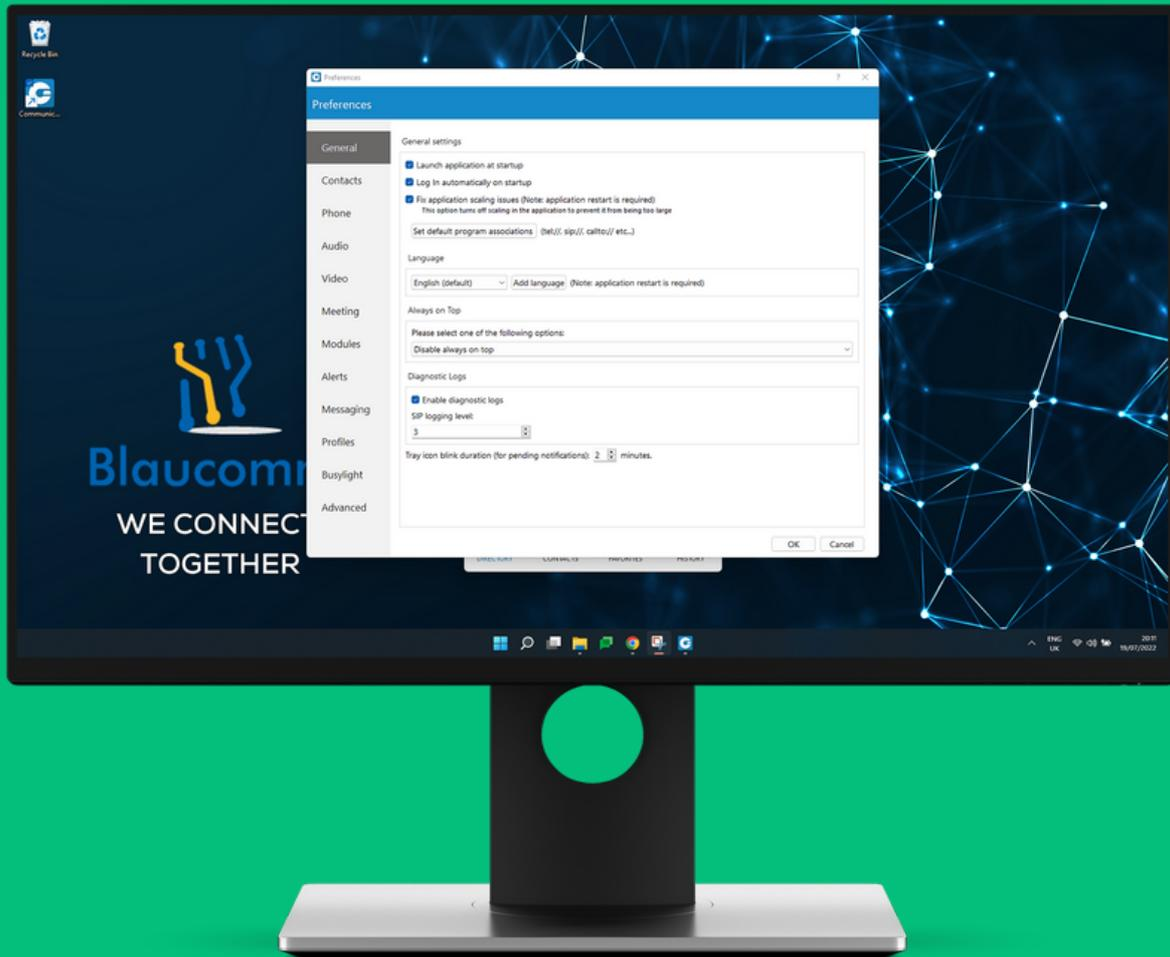
Check the boxes for **Launch application at startup** and **Fix application scaling issues**. Then click **OK**.
